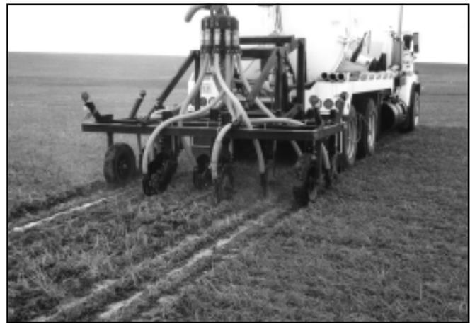
*Manure injection truck injecting 9000 gallons per acre. Note the pooling that occurs at higher injection rates.*
